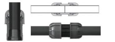
Tighten nut by hand (Tighten 32 mm and pipes bigger than 32 mm using ERHAS Coupling wrench)
